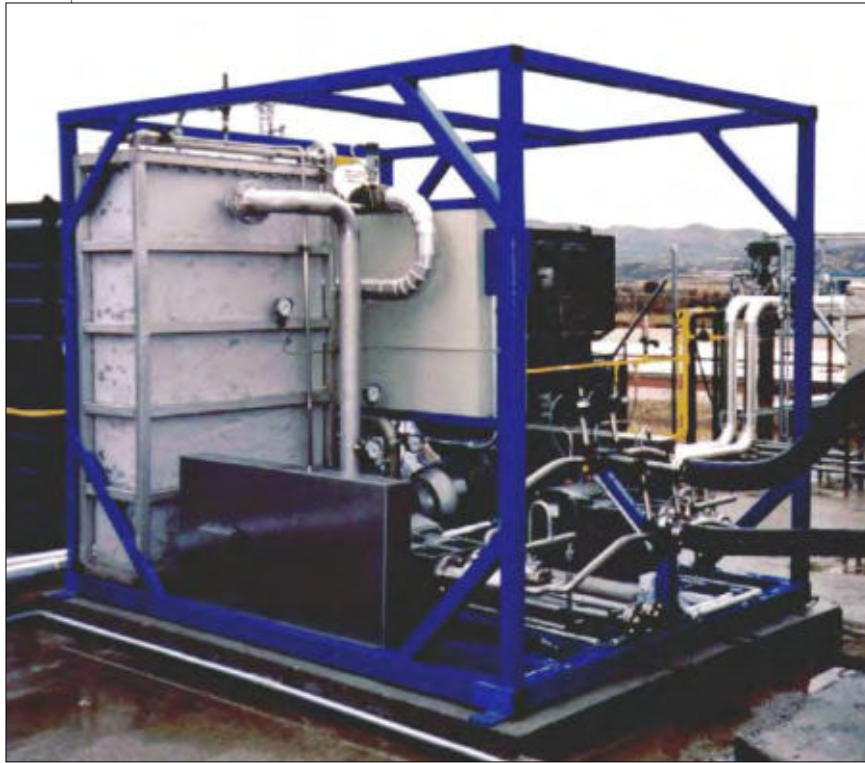
Combined O 2 /N 2 supply with PAREX evaporator 1500 Nm 3 /h, steam heated, water circulation 100 m 3 /h, (1997)
