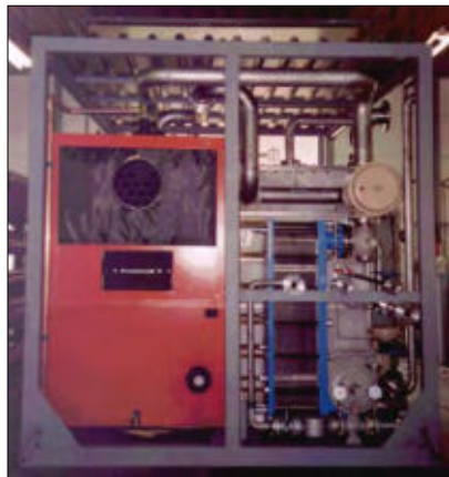
Combined O 2 /N 2 supply with PAREX evaporator 1500 Nm 3 /h, steam heated, water circulation 100 m 3 /h, (1997)
