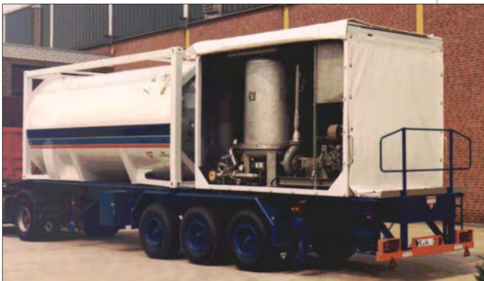
TRANSINERT plant: 4000 / 6000 Nm 3 /h N 2 (1988 / 1989)
