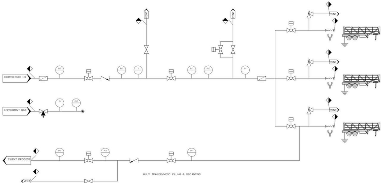
The Multi Fill & Decant configuration is a solution for sites that require both automated filling and integrated decant capability across multiple trailer/MEGC connections. Several trailers can be connected to a common module and are then processed individually through controlled sequencing.
