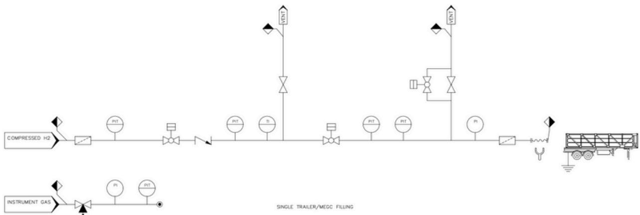
The Mono Fill configuration is a single-bay hydrogen trailer/MEGC filling solution designed for safe, repeatable operation with a high degree of automation. This configuration is particularly suitable for customers operating early-stage H<sub>2</sub> infrastructure projects that require a reliable, compliance-ready system with the ability to expand later.
