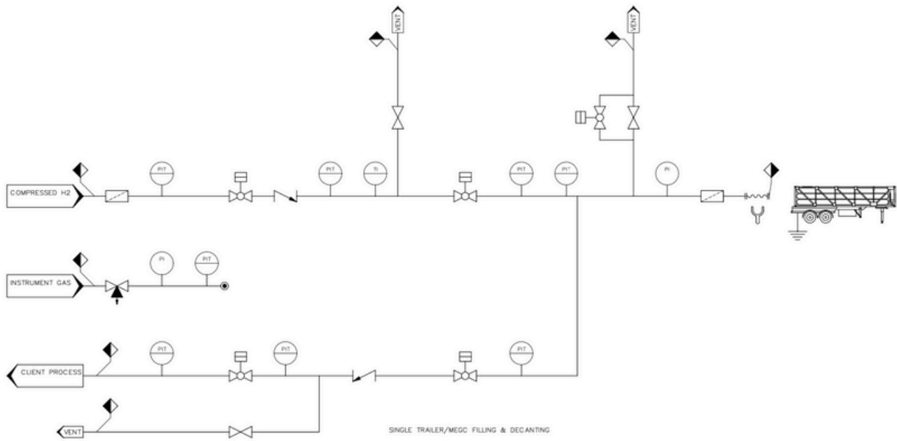
The Fill & Decant configuration combines automated trailer/MEGC filling with an integrated decant capability, enabling the system to handle both filling and controlled transfer/emptying of the trailer/MEGC depending on site requirements.
