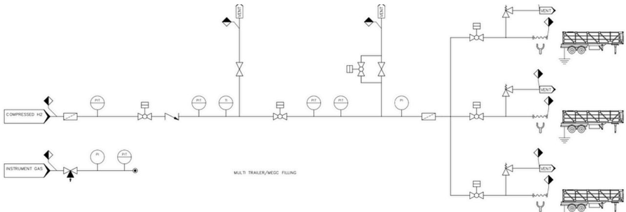
The Multi Fill configuration is a multi-bay hydrogen trailer/MEGC filling solution. Multiple trailers are connected to a common filling module and are then filled individually by controlled sequencing, supporting efficient bay utilisation while maintaining consistent safety and process control.
