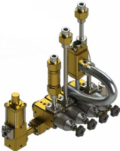
Valve modules are valves of the MPG and HPG series assembled in a manifold being interconnected at their inlet and outlet. High costs and time consuming pipe works can be avoided by this. All module bars can be connected via adapters by what different module varieties can be made up.
