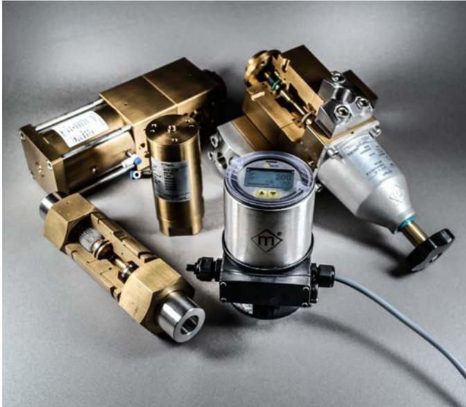
Over two decades we build our MPG series (PN420) for cylinder filling 300 bar and in 2015 we successfully launched our HPG series (PN600) for 450 bar and higher filling pressure. All our valves have been adiabatically shock tested for use with oxygen by either BAM or CTE. All components for valves are degreased and cleaned for oxygen service and assembled in our class ISO 7 standard cleanroom.
